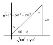
To go from a 3-D coordinate system of (x, y, z) to a 2-D coordinate system of (u, v) two rotations are made. The first is a rotation of angle  $90^{\circ} + \theta = \pi/2 + \theta$  around the z-axis and the second is a rotation of  $-\phi$  around the x-axis. The new coordinates are found by multiplying two matrices:
