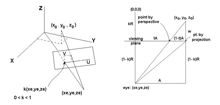
Using the common ratios in the triangle shown on the right the (u, v) coordinates are reduced by a factor of t. The distance from the point  $(x_0, y_0, z_0)$  to the viewing plane is w (assume w > 0).
